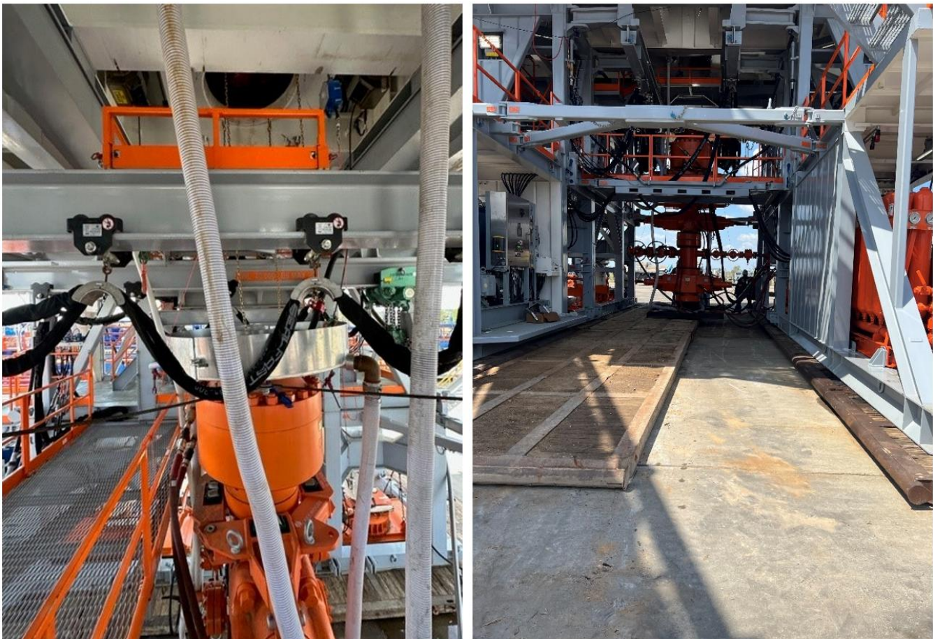
Figures 1 & 2: BOP winch system picture with walking capabilities.
