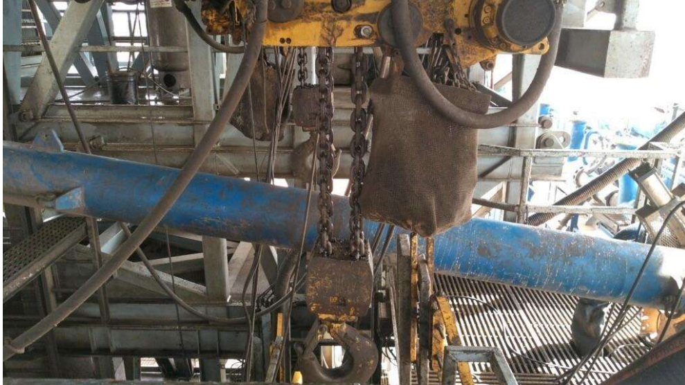
Figure 2: BOP Winch System
