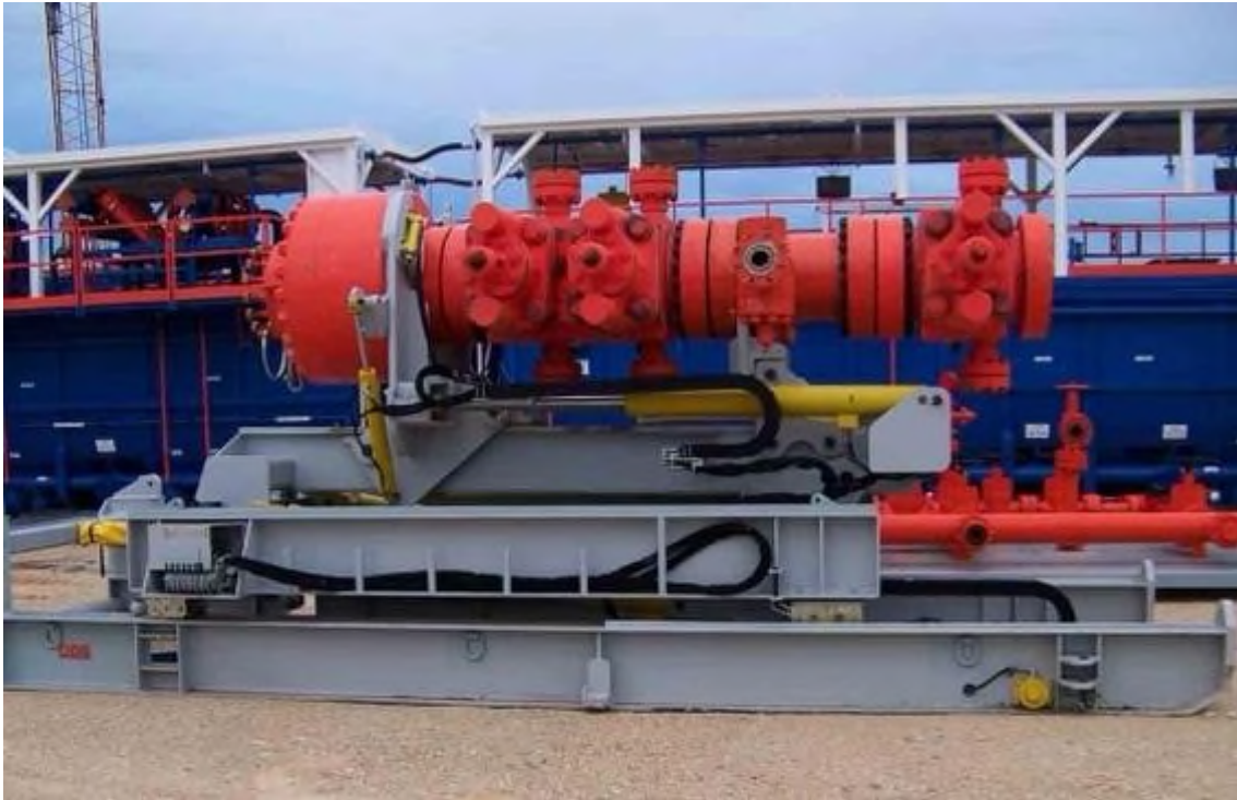
Figure 4. BOP handling system
