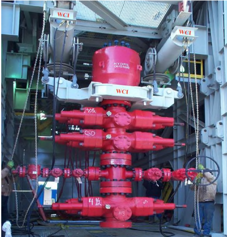
Figure 3. BOP handling system
