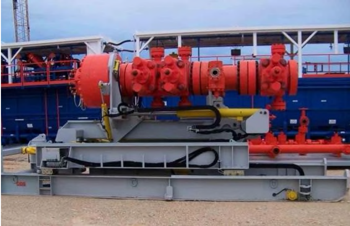
Figure 4. BOP handling system
