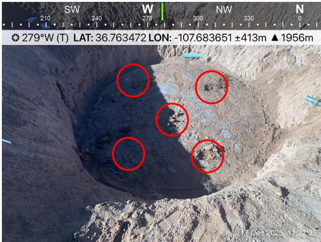
Photo 5: 5PC-TB@7'(95) is a 5-point composite sample collected below the base of the BGT following removal.
