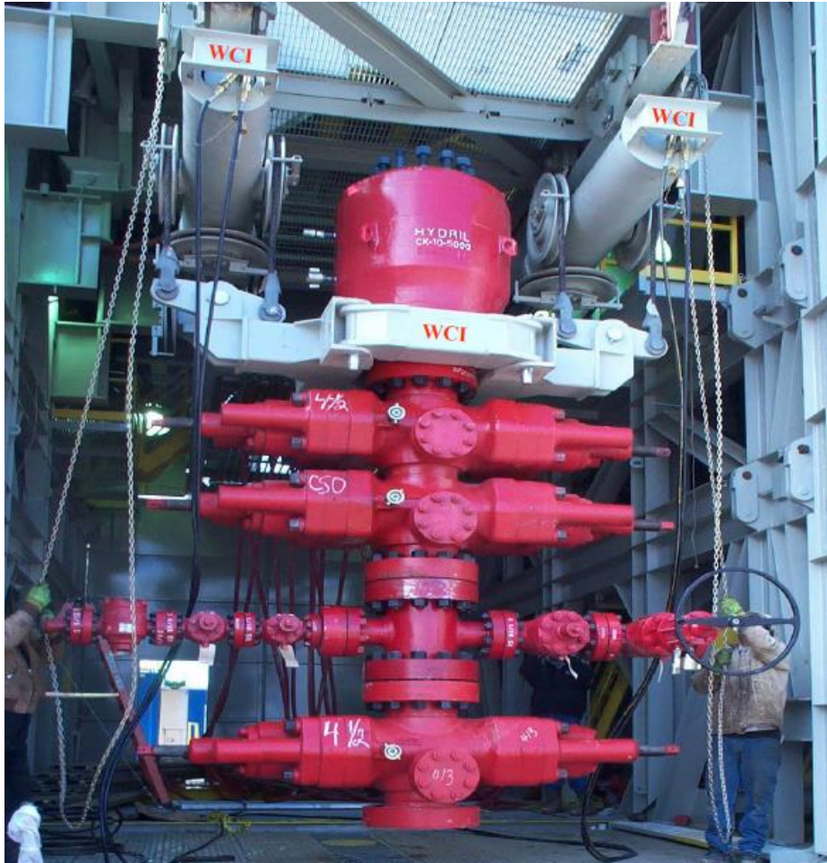
Figure 3. BOP handling system
