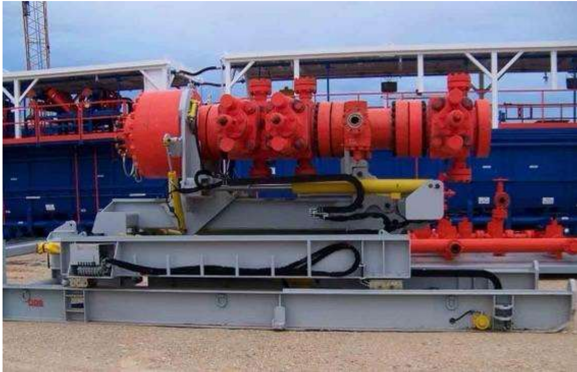
Figure 4. BOP handling system
