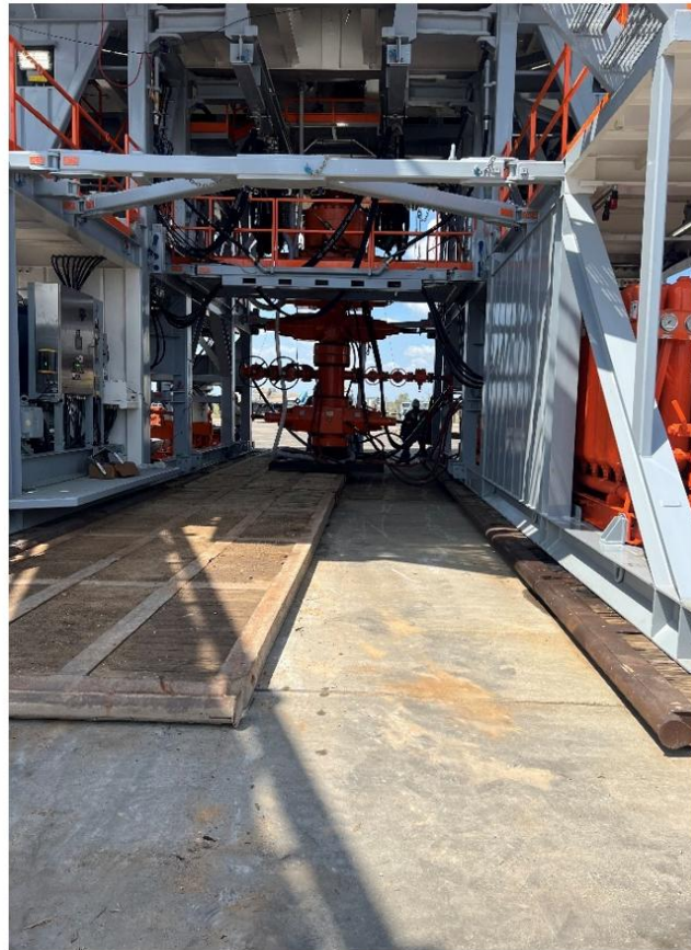
Figures 1 & 2: BOP winch system picture with walking capabilities.
