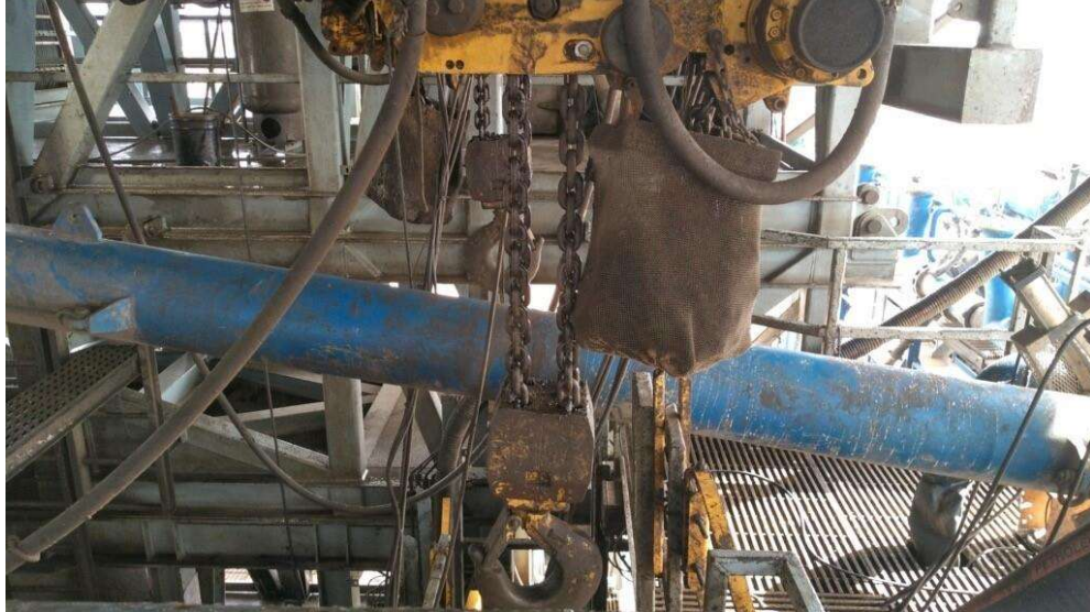
Figure 2: BOP Winch System
