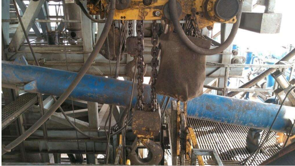
Figure 2: BOP Winch System
