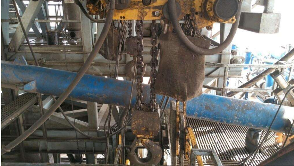
Figure 2: BOP Winch System
