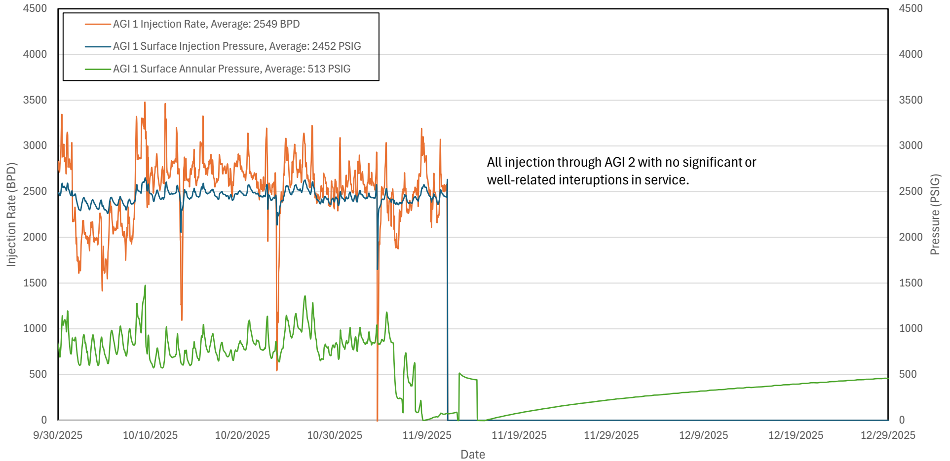
Figure 2 - Independence AGI 1 Injection Rate, Surface Injection Pressure, and Annual Pressure
