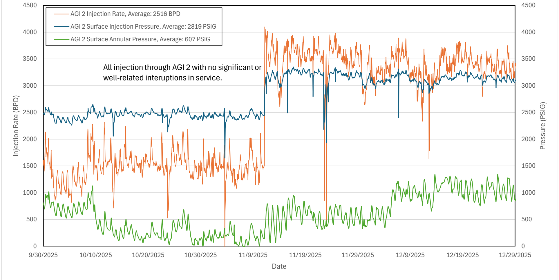
Figure 6 - Independence AGI 2 Injection Rate, Surface Injection Pressure, and Annual Pressure
