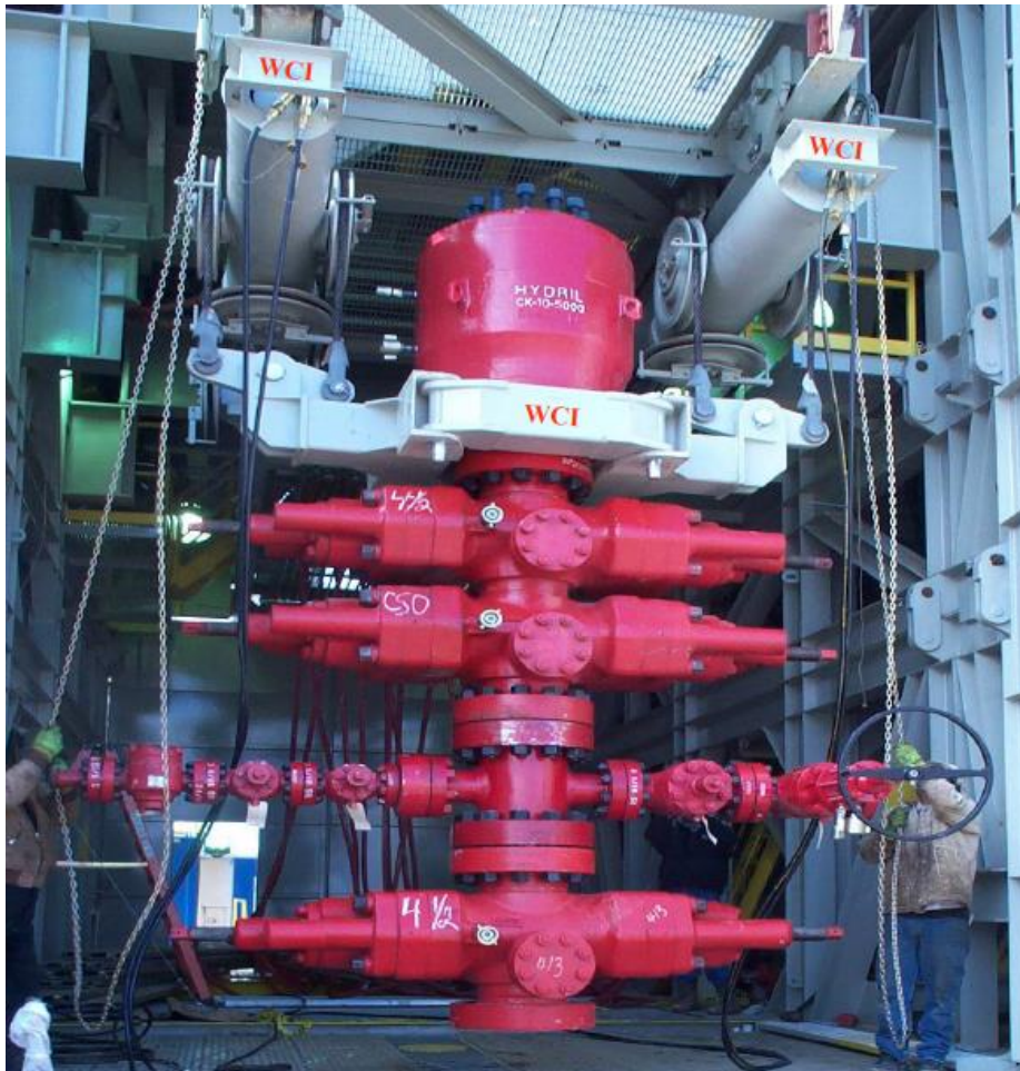
Figure 3. BOP handling system
