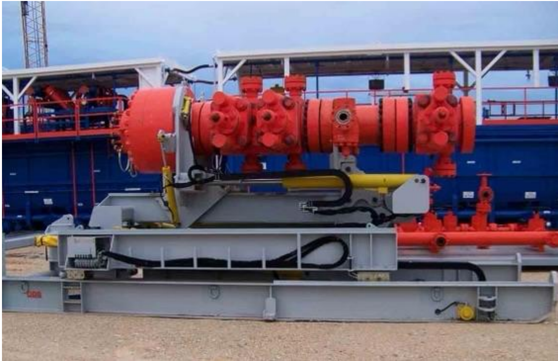
Figure 4. BOP handling system
