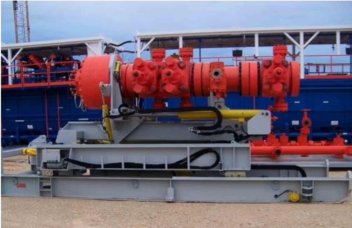
Figure 4. BOP handling system
