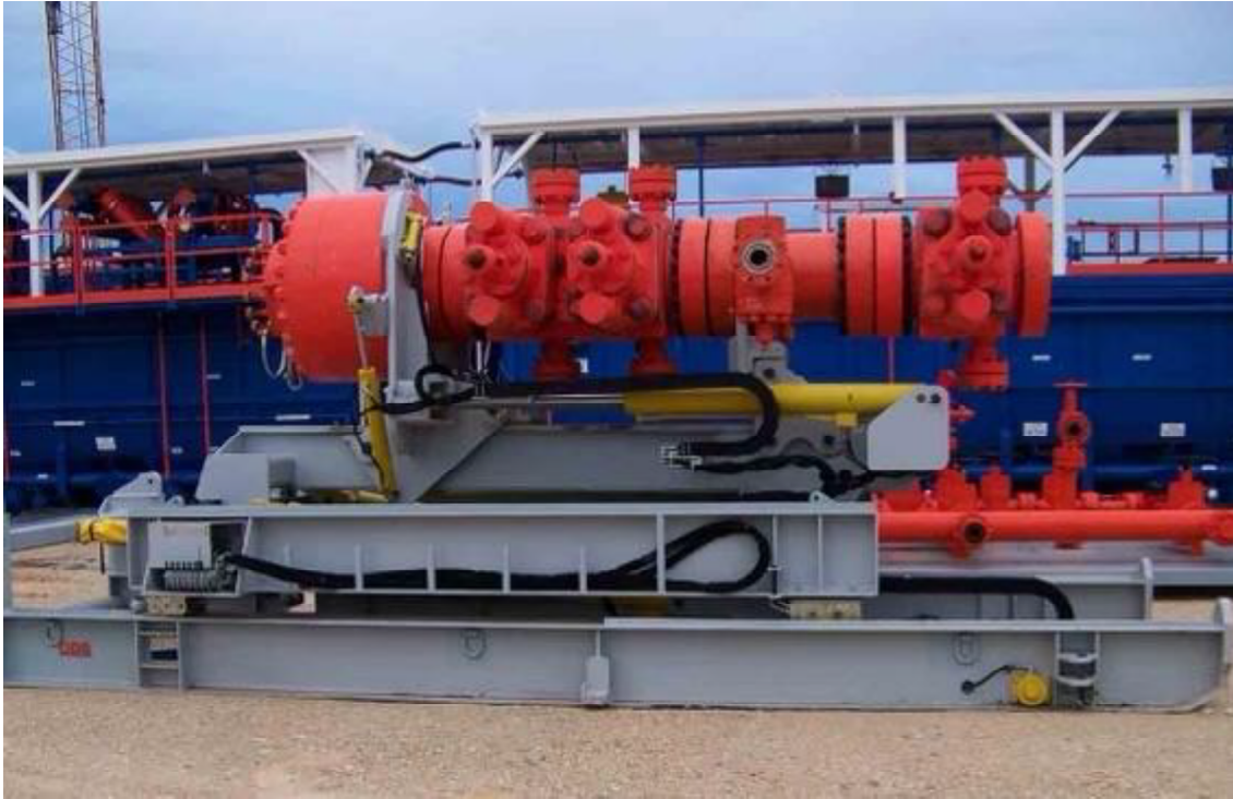
Figure 4. BOP handling system
