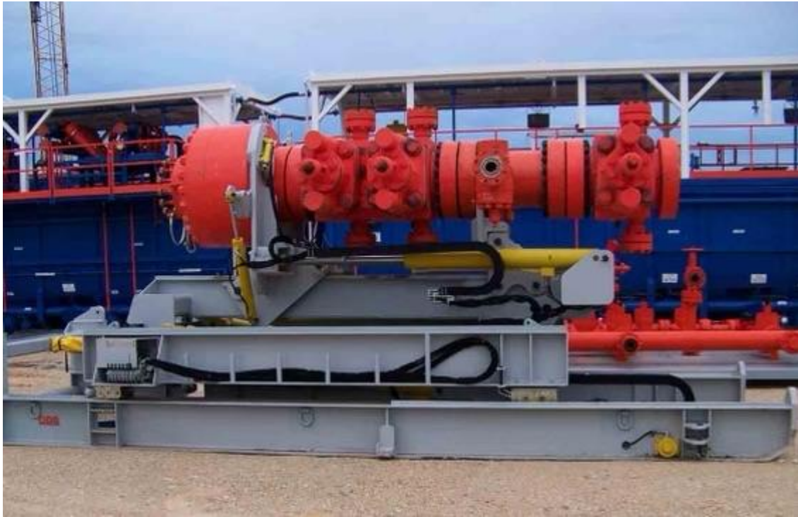
Figure 4. BOP handling system
