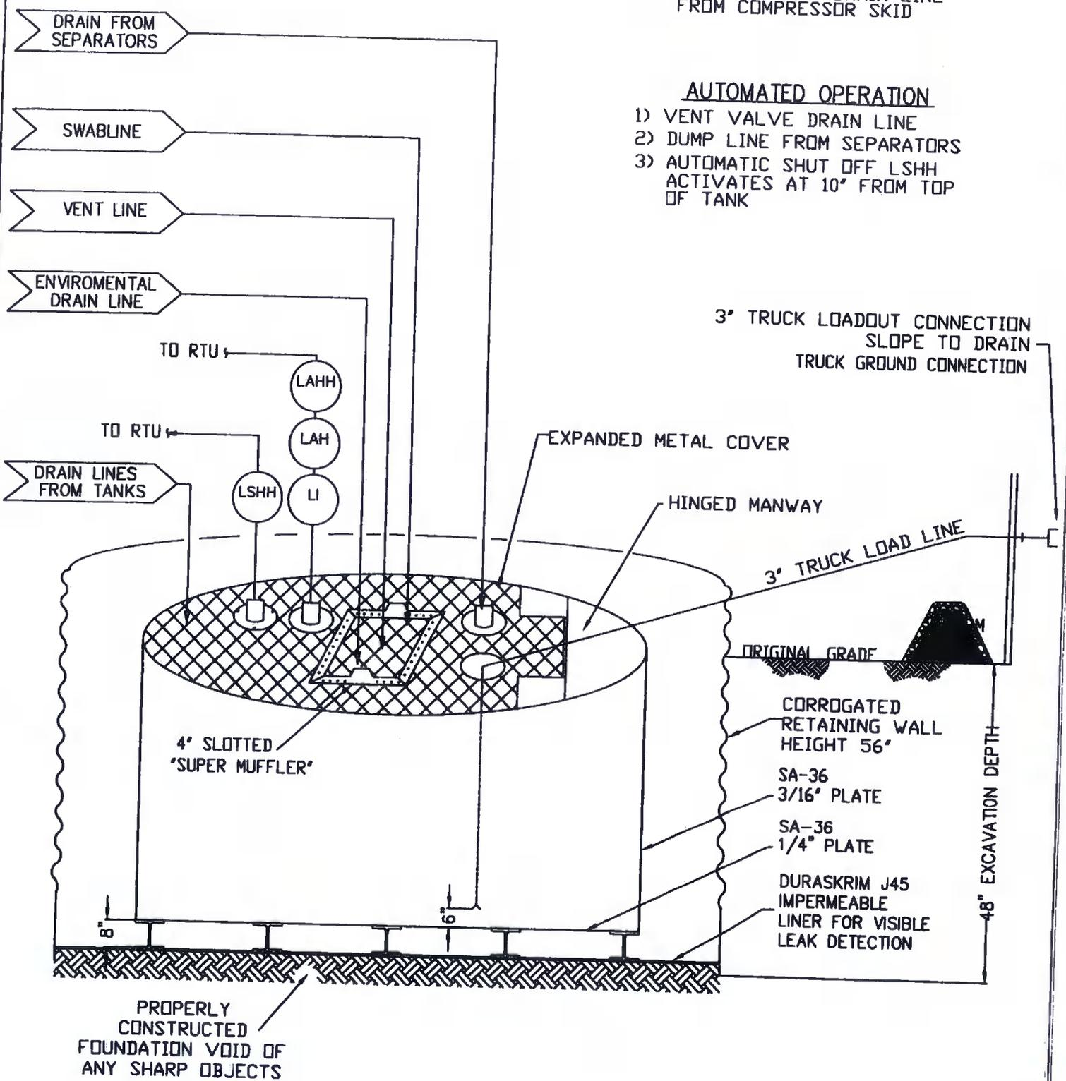
3" TRUCK LOADOUT CONNECTION
