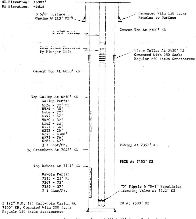
Centralizers Located 10' & 60' Above Casing Setting Depth and 90' Thereafter To 6170' KB; Also One Centralizer 30' Above & 30' Below Stage Collar.
