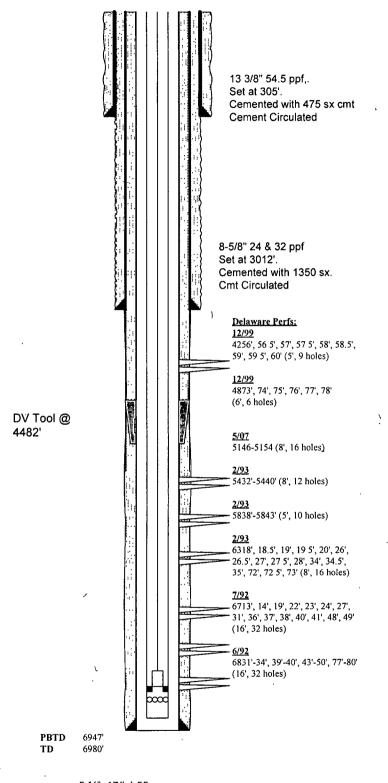
$5-\frac{1}{2}$ ", 17# J-55 Set at 6980' 1<sup>st</sup> Stage cemented with 550 sx. TOC @ 4670' below DV tool 2<sup>nd</sup> Stage cemented with 500 sx.
