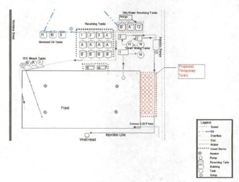
The area where the tanks will be set is flat. The 3' tall berm will serve to keep any stormwater from entering the area with the tanks.
