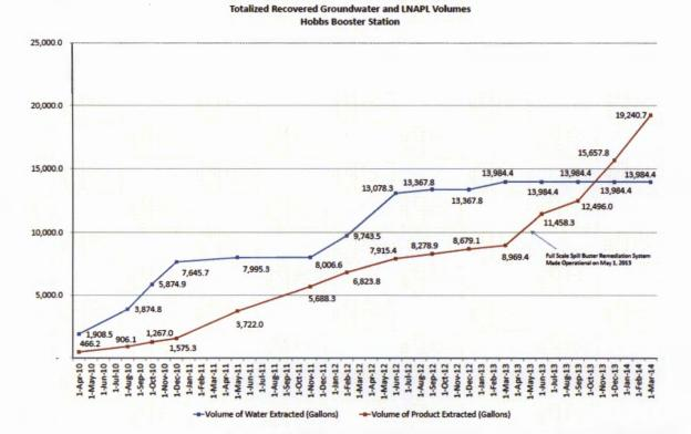
In addition to the above remediation efforts, a single solar-powered Spill Buster unit (and adjacent 500gallon poly holding tank) was operated during the first quarter 2014. During the reporting period, the solar unit was moved to MW-12 (previously deployed at MW-10). Operation at MW-12 was initiated on December 18, 2013. Between December 18, 2013 and March 28, 2014 the Spill Buster at MW-12 removed **64 gallons** of LNAPL.
