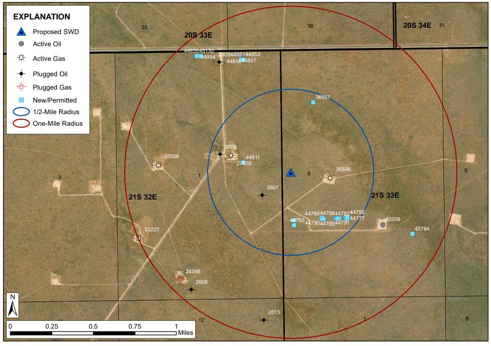
Figure A-1. All wells located within a one-mile radius of the proposed Lombard SWD #1. Well labels reflect last five numbers of API 30-0250-XXXXX and are summarized in Table A-1 of Appendix A.
