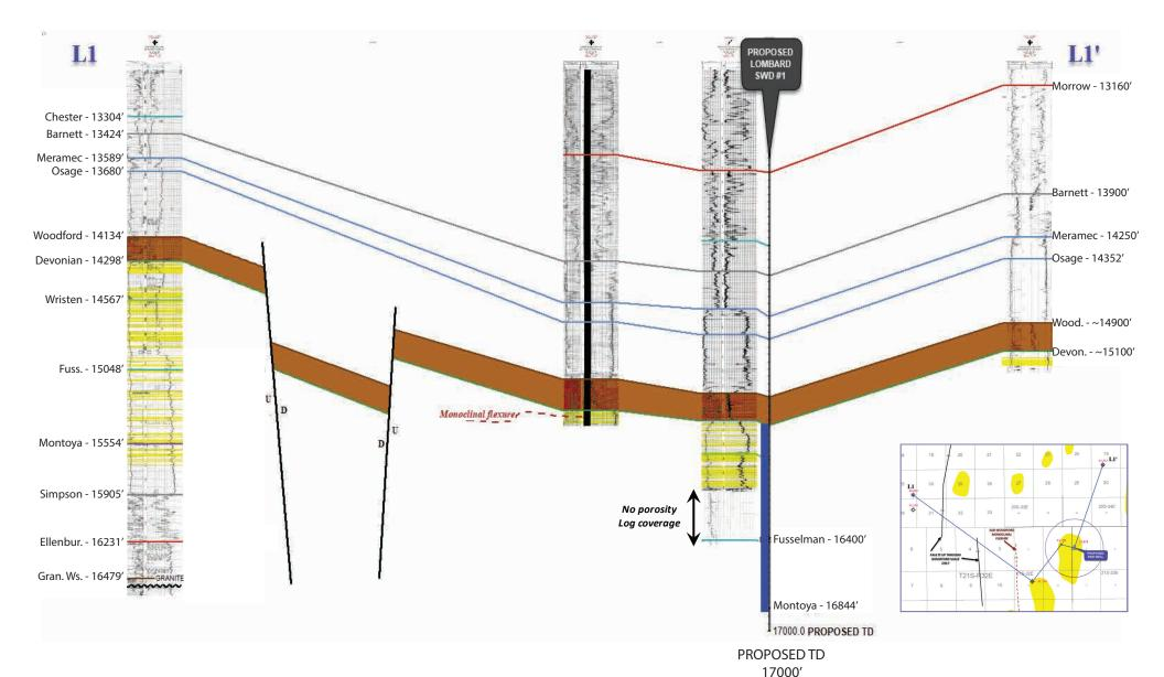
**Figure 7**. Structural cross section L1-L1' showing porosity profile within the proposed injection interval and regional extent of overlying caprock material. Two faults were identified in the area of the proposed Lombard SWD #1 and are discussed in greater detail in Section 4.6.
