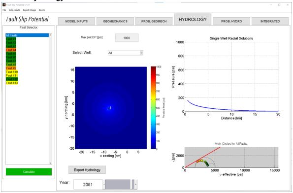
Year 30 Probabilistic Hydrology (note no crossover between blue delta-press. & green fault slip press.)
