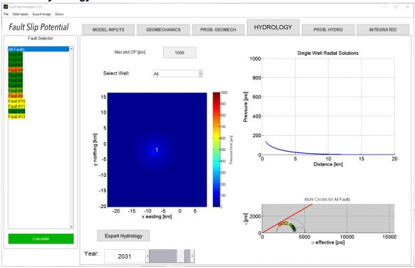
Year 10 Probabilistic Hydrology (note no crossover between blue delta-press. & green fault slip press.)
