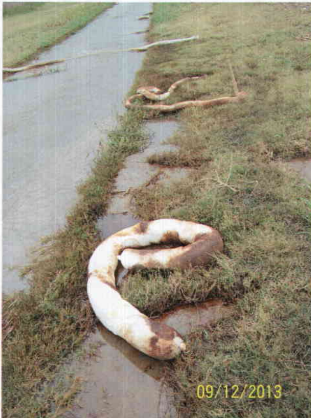
Cleaning oil from eddies. Current in concrete swale pushed oil into eddies on the outer curve, making it easier to collect and capture
