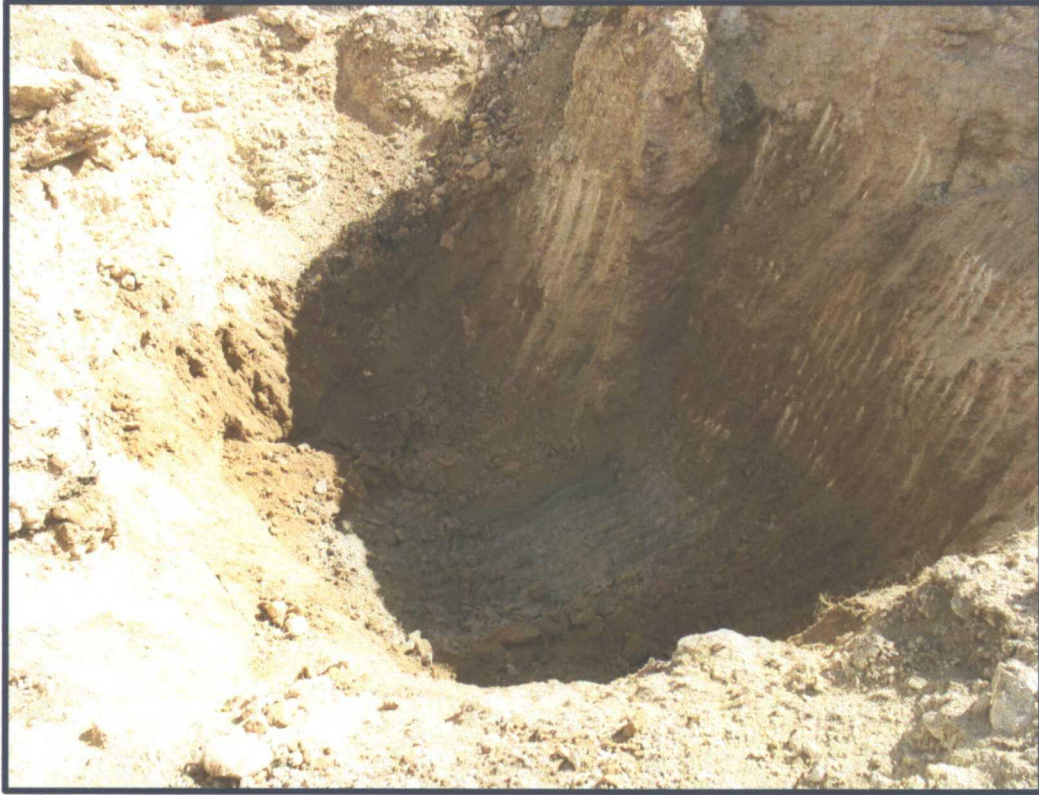
Photograph #7: View of color change in excavation area S-1 at a depth of approximately 20 feet bgs.
