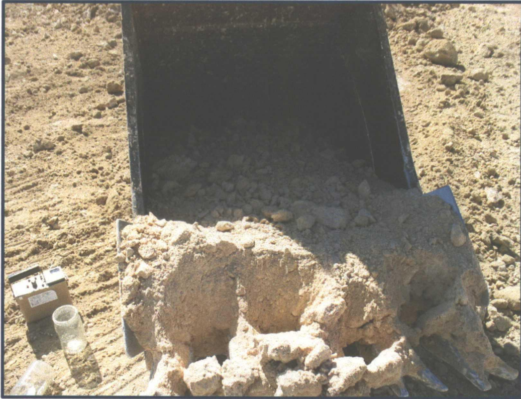
Photograph #17: Close-up of material excavated from pot-hole area S-4 with scintillator to left of excavator bucket.
