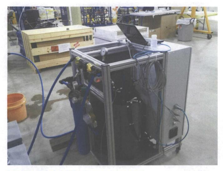
Figure 3. Voltea CapDI system (as installed for brackish water desalination experiments)
