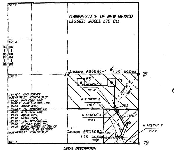
A STRIP OF LAND 30.0 FEET WIDE, LOCATED IN SECTION 18, TOWNSHIP 17 SOUTH, RANGE 29 EAST, N.M.P.M., EDDY COUNTY, NEW MEXICO AND BEING 15.0 FEET LEFT AND RIGHT OF THE FOLLOWING DESCRIBED CENTERLINE SURVEY.
