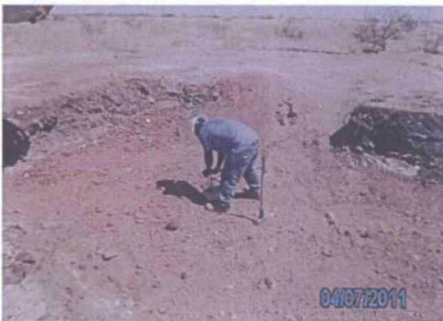
Compaction test on clay liner, facing north 4.7.11
