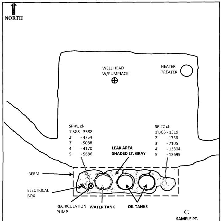
surface of spill area west end very black, oily, dirt mixed w/caliche, material remains the same up to the east tank then starts to change in color. Area of sp #2 possible area of past tank, and a gathering area for any run off to gather and puddle. Signs of where water did gather and was vacuumed out in area. samples were hand augered from 1'bgs to 5'bgs
