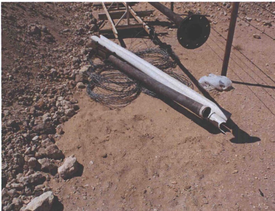
4 Inch PVC Line and Dresser Sleeve from West Excavation, March 22, 2011
