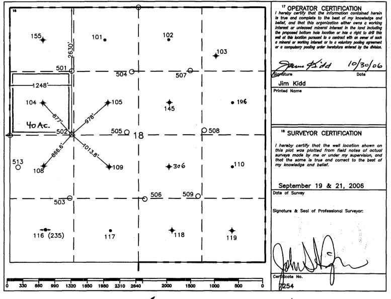
° = Staked Location • = Producing Well 🔊 = Injection Well 📀 = Water Supply Well 🔶 = Plugged & Abandon Well  $\odot$  = Found Section Corner, 2 or 3" Iron Pipe & GLO B.C. o = Found /4 Section Corner, 1" Iron Pipe & GLO B.C.
