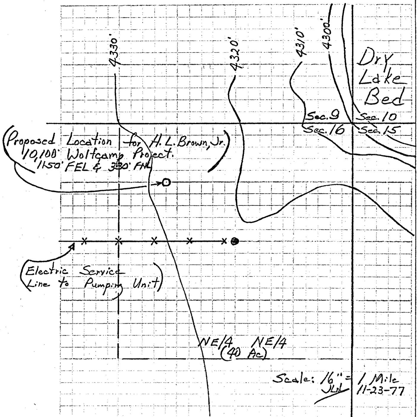
PLAT SHOWING UNIT "A" OF SECTION 16, T-16-S, R-32-E, LEA COUNTY, NEW MEXICO, WITH TEN (10) FOOT CONTOURS ON THE TOPOGRAPHY AND LOCATION OF ELECTRIC SERVICE LINE. SURFACE IS COVERED WITH FEW INCHES OF SOIL AND UNDERLAIN WITH SOLID CALICHE
