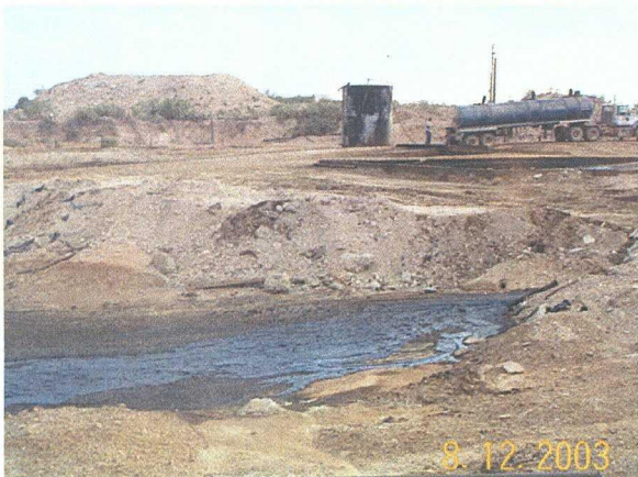
Photo 3: Warm water returning from the centrifuge process to Pond 4.
