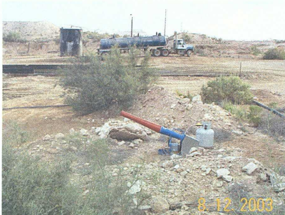
Photo 2: Propane cannon used to scare the birds, southeast corner of Pond 4.
