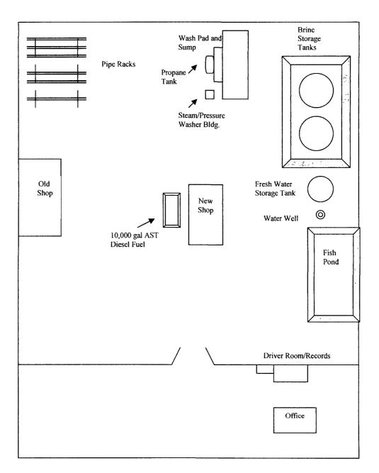
Note: Brine Storage Tanks are bermed with liners for leak protection; Fish Pond is unlined with berms.
