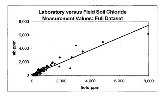
Field soil chloride measurement thus provides a reasonable surrogate for laboratory measurement (which may be presumed to be closer to the true values), and the ability to distinguish between low and high levels of chloride contamination.
