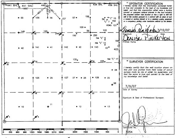
O = Staked Location • = Producing Well = Injection Well • = Water Supply Well • = Plugged & Abandon Well () = Found Section Corner, 2 or 3" Iron Pipe & GLO B.C. () = Found /4 Section Corner, 1" Iron Pipe & GLO B.C.
