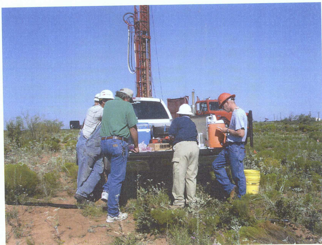
View facing west showing chloride screening activities for soil samples obtained from monitoring well MW-1 at the Santa Rita EOL site (08-30-05)
