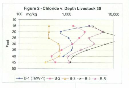
materially impact the lower vadose zone in the north of the former pit (note that borings 2 and 3 were not drilled within the former reserve pit). In the central and southern portion of the excavation (within the area of the former reserve pit), chloride concentrations above the capillary fringe are 1,298 mg/kg (B-1), 2,799 mg/kg (B-4) and 2,031 mg/kg (B-5).
