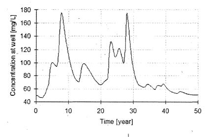
Figure 7. Simplified simulation of a 2-foot thick chloride mass of 2,300 mg/kg placed 18 feet above ground water.
