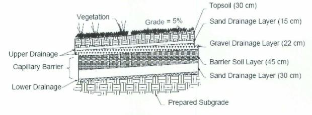
Profile of Alternative Test Cover 3 (Landfill 5)
