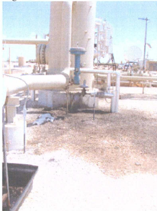
Photo 26 : Sulfur unit with discharge on ground.
