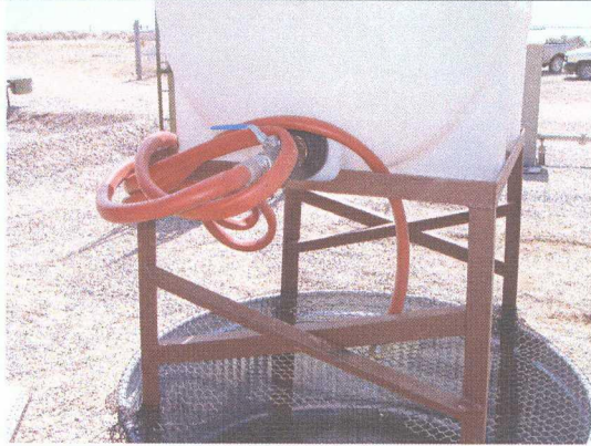
Image 7: Reconfigure extruding plumbing of saddle tank to prevent discharge on to ground of hose.
