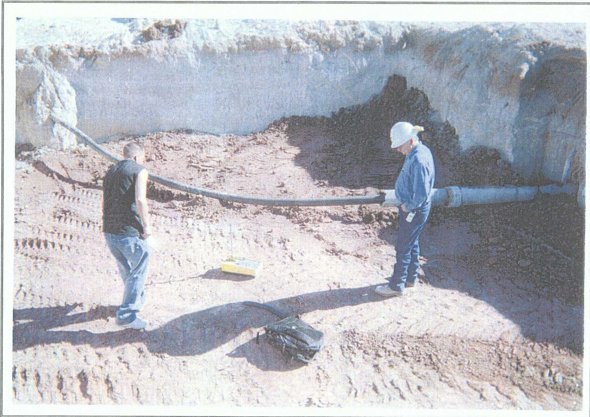
9. Nuclear density test being performed on clay liner.
