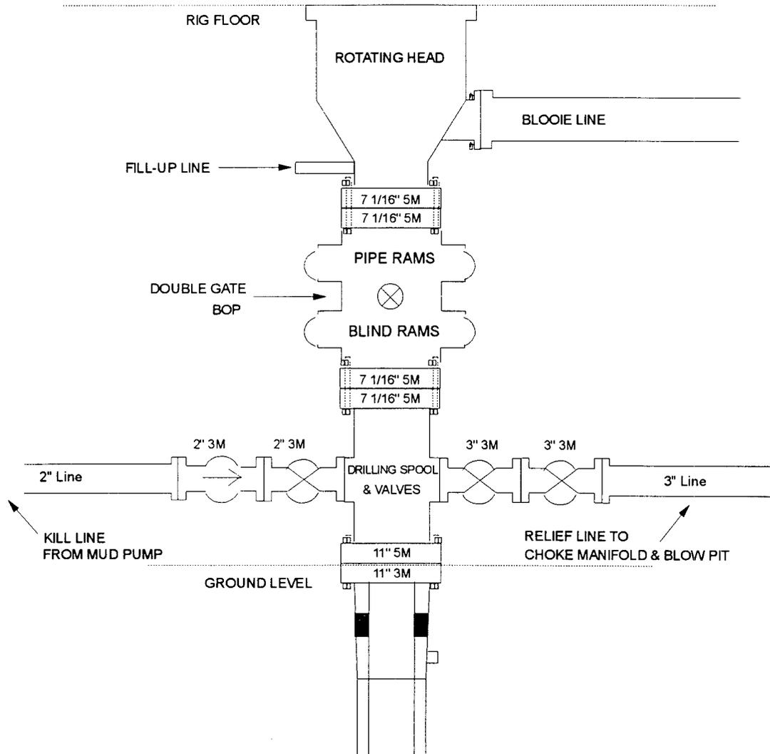
Minimum BOP installation for Completion Operations. 7 1/16" Bore (6" Nominal), 5,000 psi minimum working pressure double gate BOP to be equipped with blind and pipe rams.
