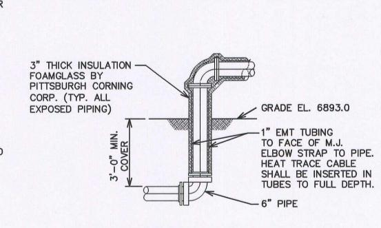
**EMERGENCY TANKS** DRAIN DETAIL SCALE: 3/8" = 1'-0"
