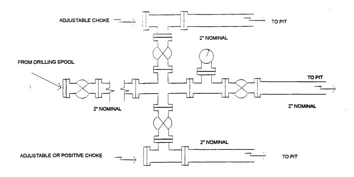
Minimum choke manifold installation from surface to Total Depth. 2" minimum, 2000psi working pressure equipment with two chokes.
