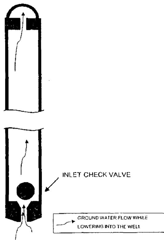
FIG. 2 Single Check Valve Bailer
