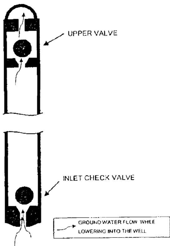
FIG. 3 Double Check Valve Bailer
