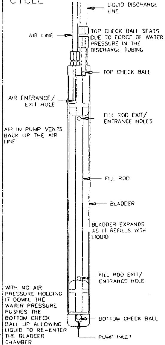
FIG. 4 Squeeze Type Bladder Pump
