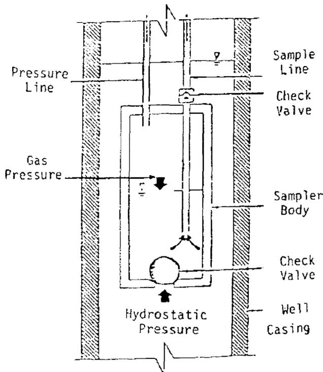
FIG. 5 The Principle of Gas Displacement Pumping
