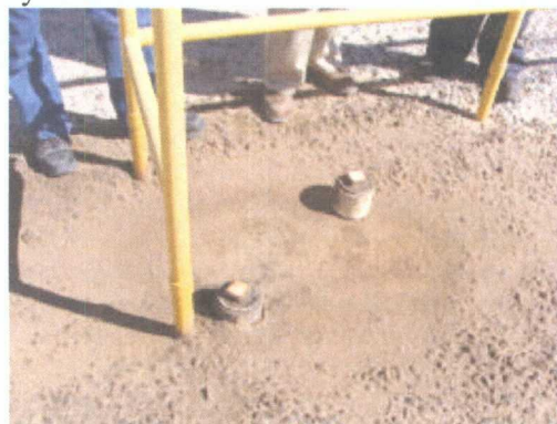
Photo 11: Ports with soil staining near water tanks, assume gasoline.
