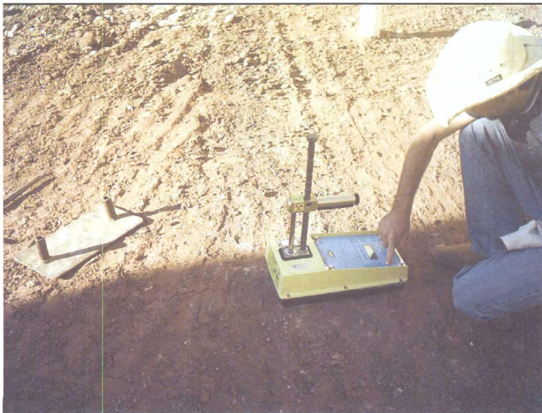
Photograph 12: Pettigrew & Associates P.A. (Pettigrew), a qualified engineering firm, tested each one foot thick layer of compacted clay.
