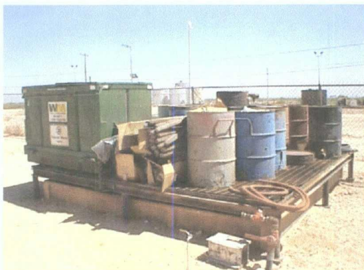
Pic#3 Special waste area with secondary containment.
