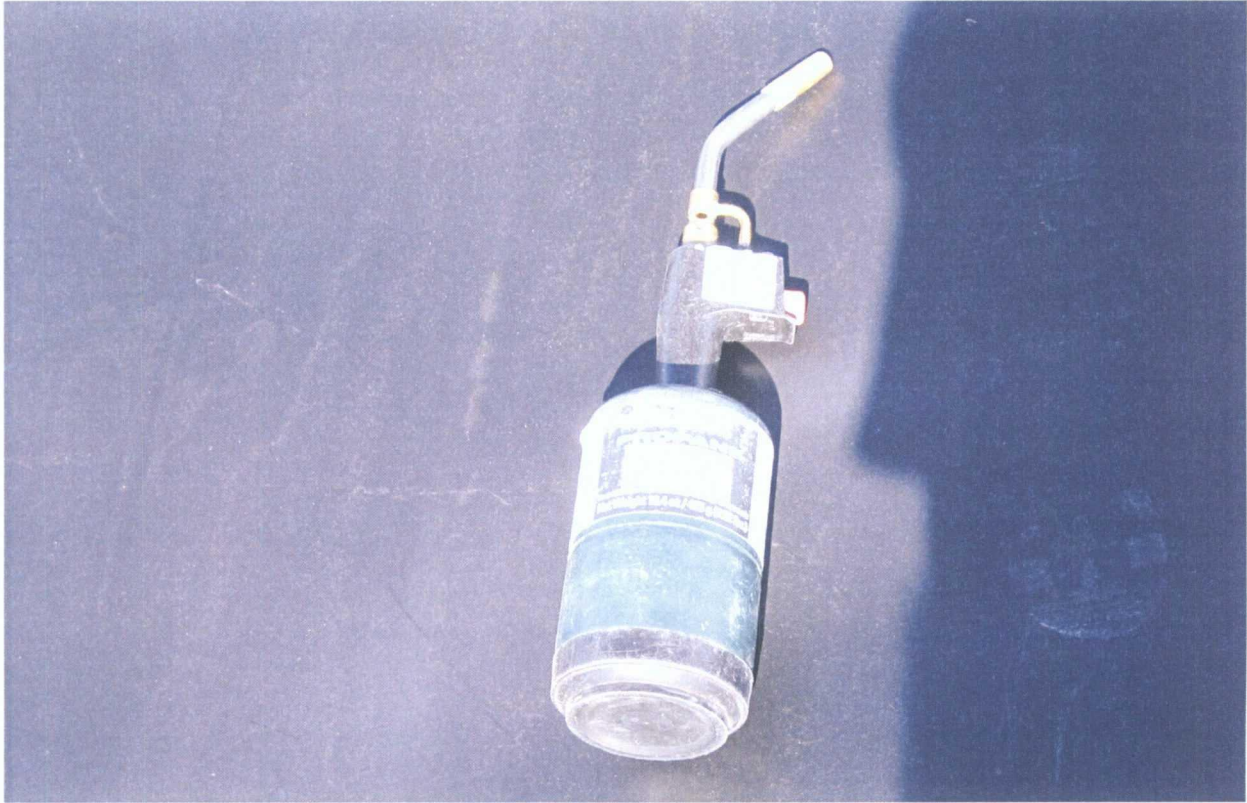
26. 6-16-09 Torch used for seaming wedge welds to do air pressure tests
