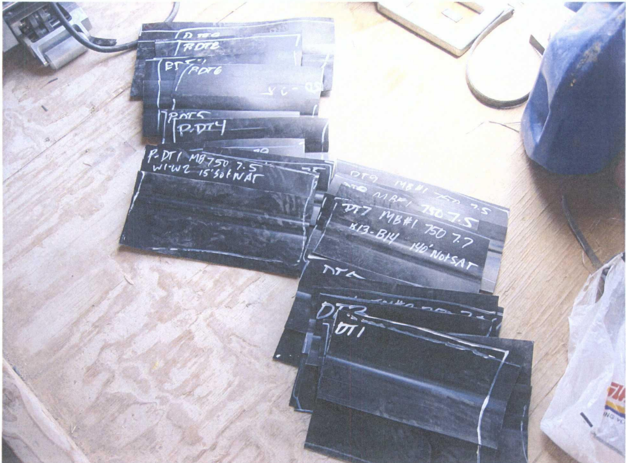
66. 6-23-09 Owners DT samples, both secondary (noted as DT) and primary (noted as PDT) HDPE liners
