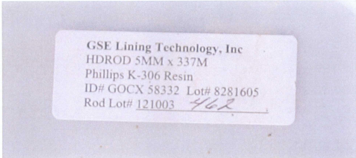
30. 6-16-09 Manufactures tag on extrusion welding rod
