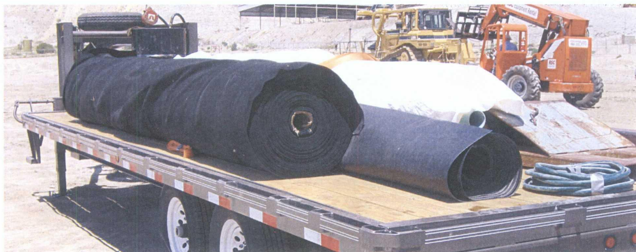
18. 6-15-09 GCL, Geotextile and Textured FML
