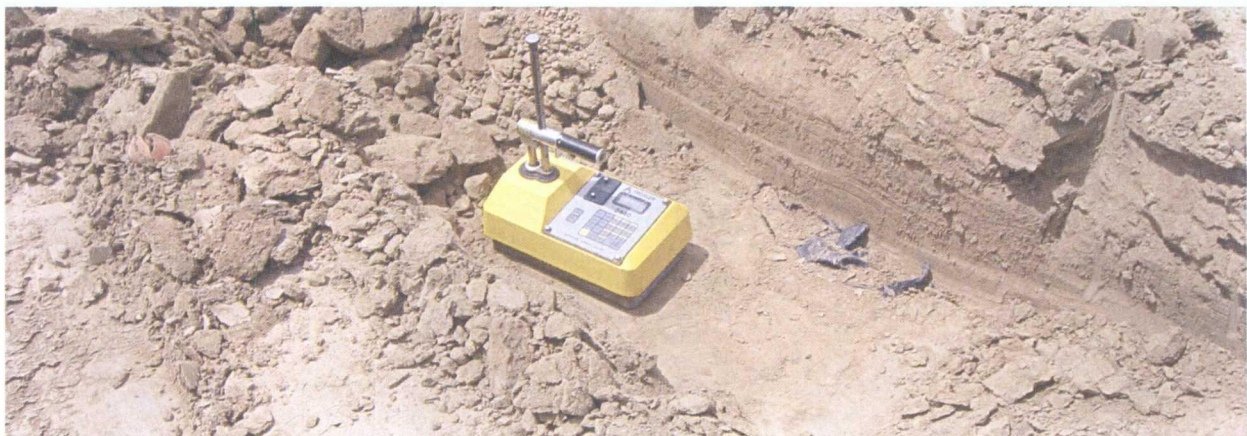
7. 6-1-09 Density testing on 1 st of two lifts constructed
