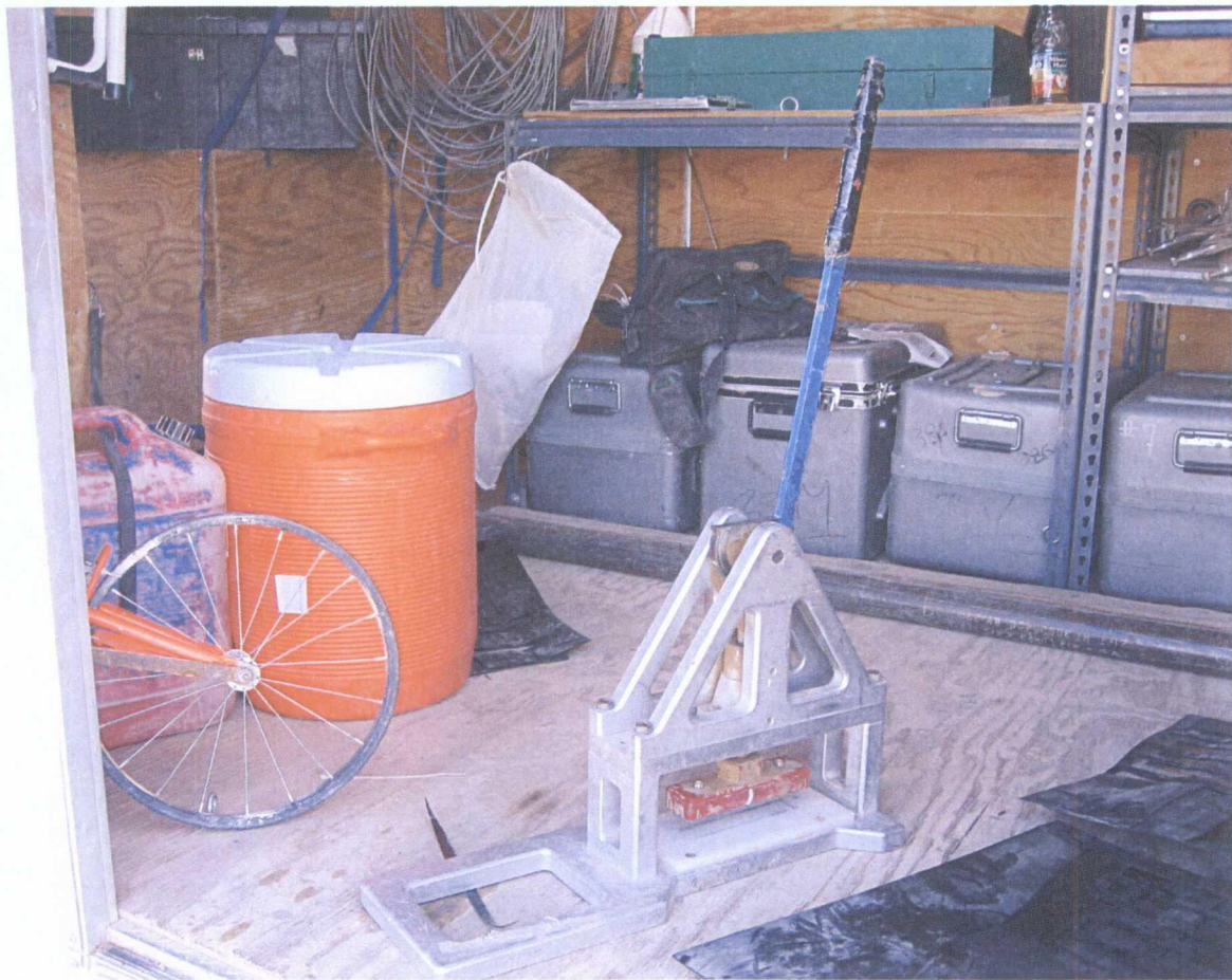
31. 6-16-06 Punch used for cutting destructive tests and pre-weld tests
