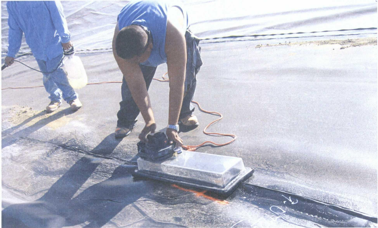
69. 6-24-09 Vacuum testing extrusion welds
