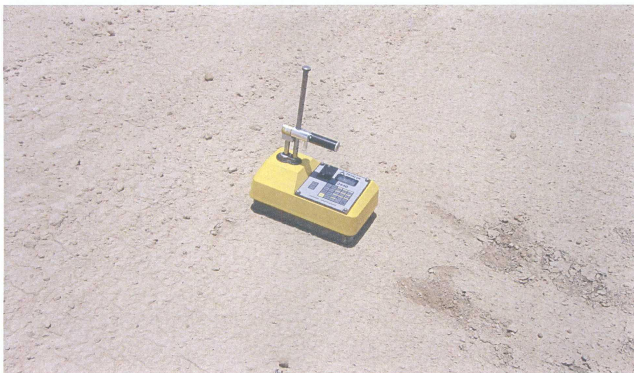
9. 6-9-09 Density testing the sideslope of Evaporation Pond 3
