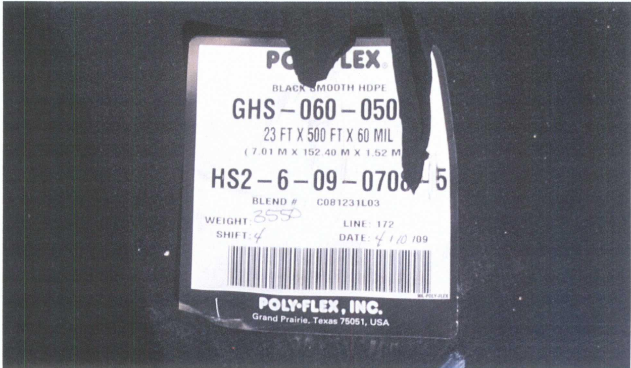
24. 6-16-09 Manufacturer roll number identification
