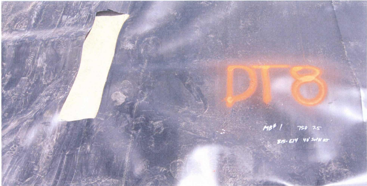
40. 6-17-09 Secondary liner Destructive Test (DT) cut and ready for patching
