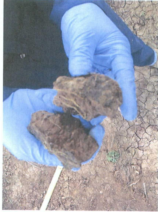
Photo 19. B8 - Black staining broken (not evident on fresh surface)
