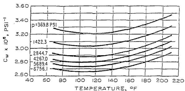
Fig. D.16 Average compressibility of distilled water. After Long and Chierici.<sup>13</sup>
