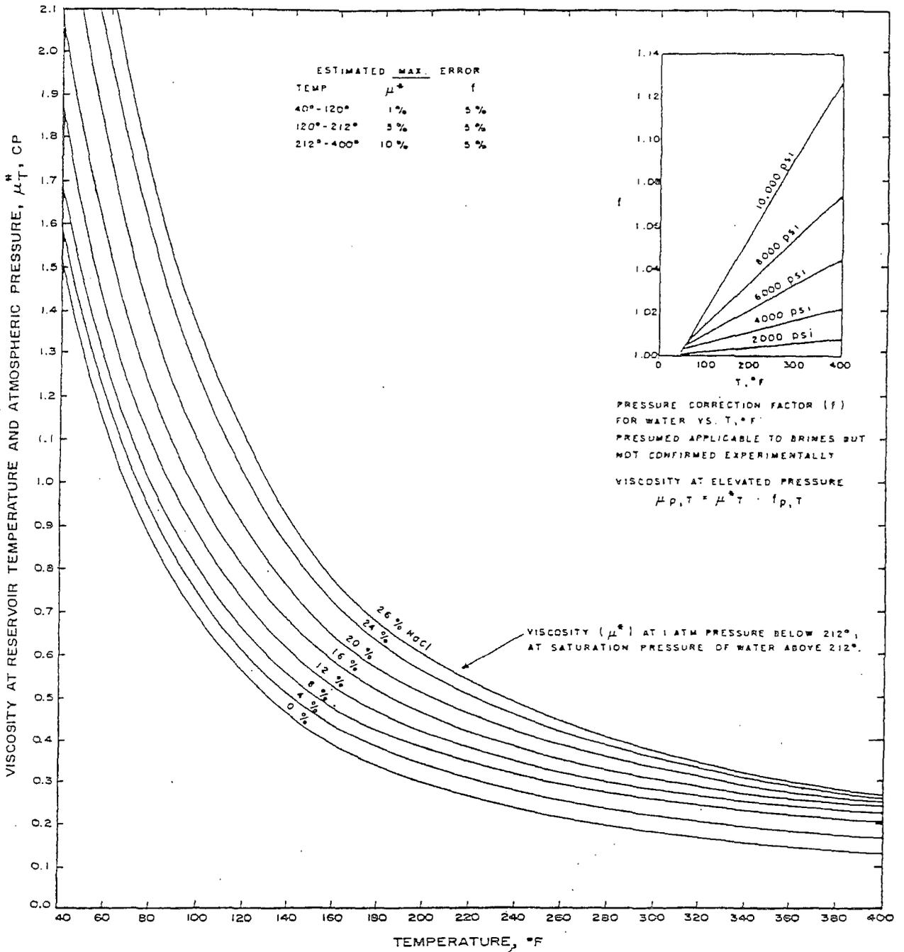
Fig. D.35 Water viscosity at various salinities and temperatures. After Matthews and Russell, data of Chesnut.<sup>18</sup>
